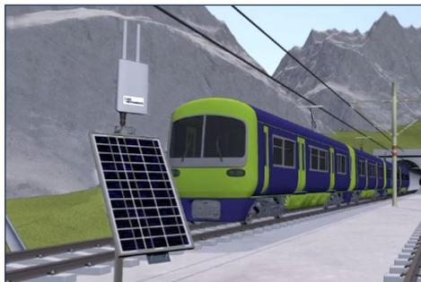
A cellular gateway collects the readings and transmits them to the internet. Gateways can be powered by a solar panel or AC mains. Costs for deploying this system are much lower than with cabled sensors.
