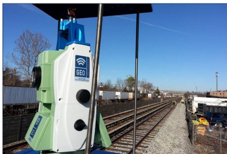
This AMTS was one of an array of fifteen used to monitor potential deformation of the track over a 2.5 mile span.
