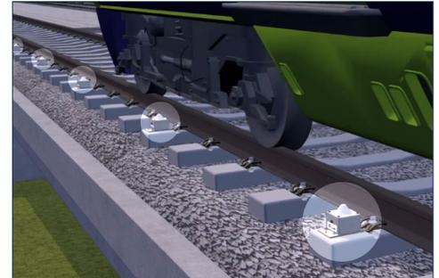
Wireless mesh tiltmeters are fixed to the ties with screwed in brackets or with glue. Each tiltmeter relays its readings to a neighboring tiltmeter. This allows transmission around curves and obstructions.
