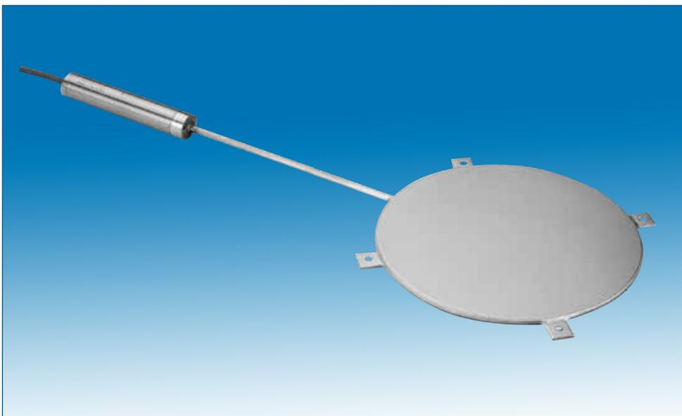
**Earth pressure cells** are sensitive on both sides. They are embedded in fills, sometimes in arrays with each cell in a different orientation.
