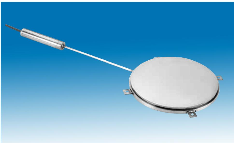
**Contact pressure cells** are sensitive on just one side. The other side is a rigid back plate which is fixed to a structure.
