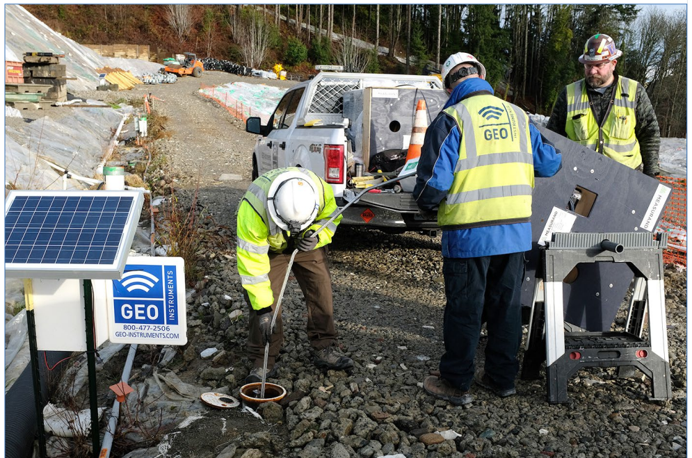
Deploying a shape array, also known as an SAA - Shape Accel Array.
