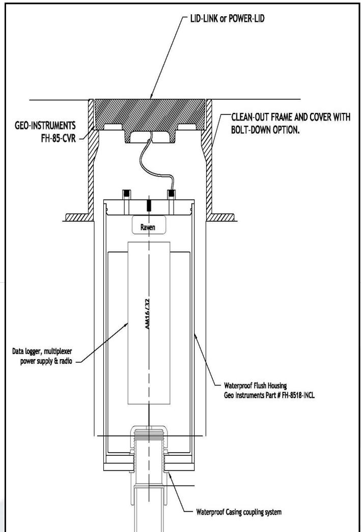
Above: Typical Subsurface Wireless IPI installation with LidLink.
