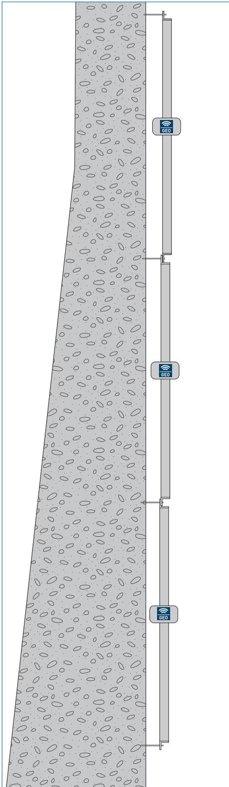
Fixed inclinometer with 3 segments
