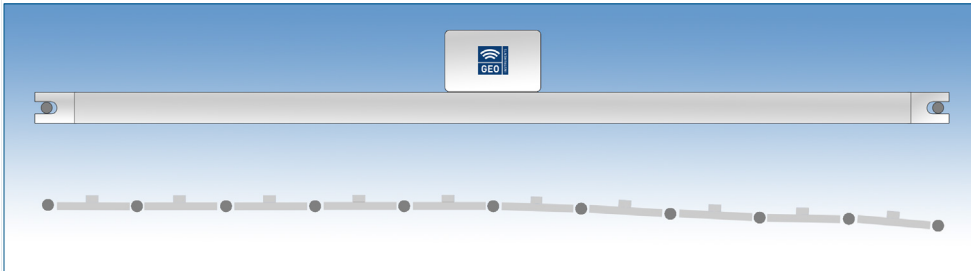
Tiltmeters mounted on beams can be used to monitor differential settlements
