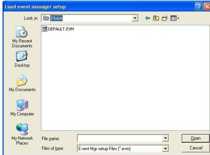
Select a setup file. All setup files have an .evm extension and appear in Blastware’s dbase subdirectory. Click **OK** to load the file. To exit without loading a setup file, click **Cancel**.
