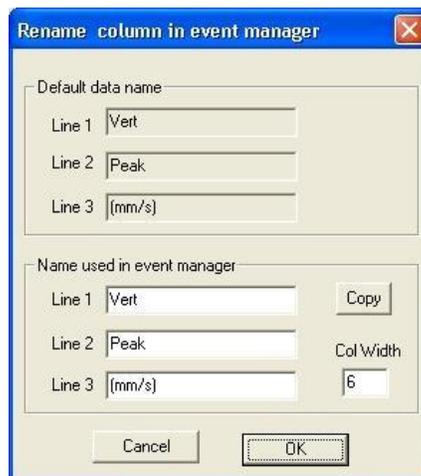
The dialog box presents two sections. The first section, Default data name, displays the default Instantel column name. The second section, Name used in Event manager, displays the names currently used. These names can be changed. Names can be entered on Lines 1, 2, 3, or all. Names may include alphanumeric characters. You can specify the width of the column by entering the
