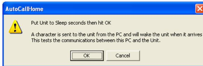
i Click OK on the new dialog that appears. The unit will turn on and display a “Connecting” message. If the unit does not wake up within 20 seconds, the follow the directions on this dialog:
