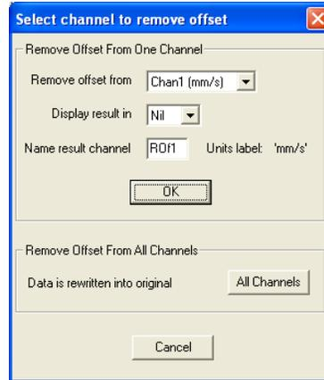
Choose a waveform to remove the offset in the first drop-down menu. In the second drop-down menu, choose a waveform window to display the new waveform. Lastly, name the new waveform. Press **OK** to create the new waveform. If you would like to remove the offset from all of the channels, click on the **All Channels** button.
