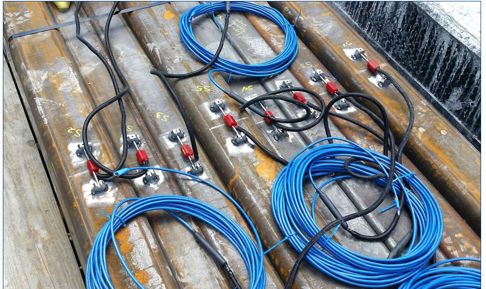
Struts instrumented with arc-weldable strain gauges
