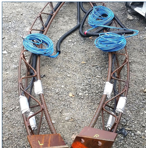
Careful positioning of the strain gauges on these lattice girders along with protective metal-foil wraps yielded a 100% survival rate during shotcreting.
