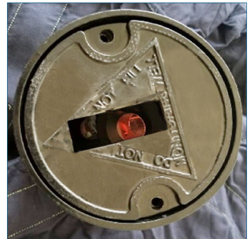
Well cover with slot for prism.
