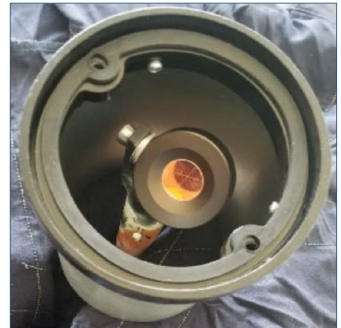
Prism fitted to top of riser.
