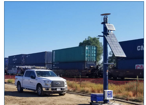
AMTS systems mounted on towers can be positioned nearly anywhere for best lines of sight. Solar panels provide power.
