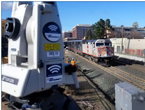
This AMTS system is monitoring rail clip prisms on the tracks and road prisms on a road crossing.
