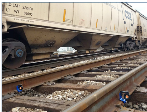
Prisms are typically installed on both rails.
