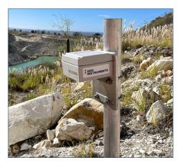
Tiltmeters can be mounted on stakes or poles and used to trigger alarms when sudden movement occurs.
