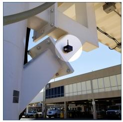
Airport jetbridge monitored by wireless tiltmeter during adjacent foundation work.
