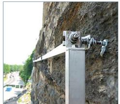
Tiltmeters can be installed on vertical or horizontal arrays of beams to monitor differential settlement and deformation.
