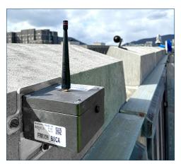
Tiltmeters can be mounted on structures to monitor stability. Brackets are available for nearly every environment.
