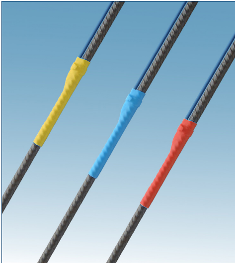
Sister bar strain gauges set to measure compression (yellow), midrange (blue), and tension (red).
