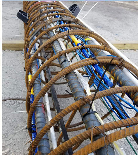
This rebar cage is instrumented with both sister bar strain gauges and thermal wires for TIP testing.
