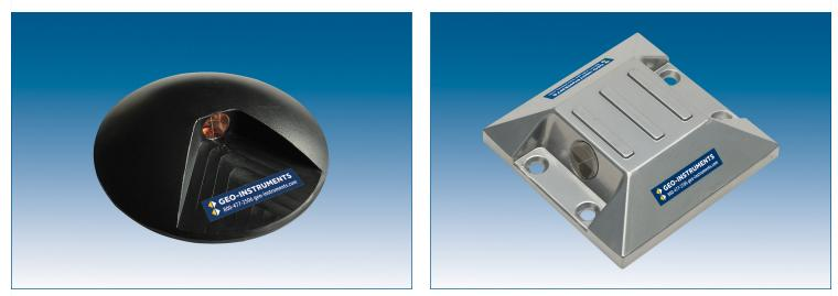
Road prisms are low-profile optical targets used with AMTS to monitor settlement and deformation of roads, pavement, and other surfaces. GEO-Instruments offers a polymer version and a cast-aluminum version.
