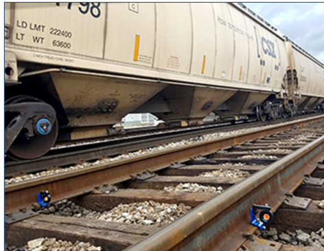
Paired Prisms Monitor Changes in Cant
