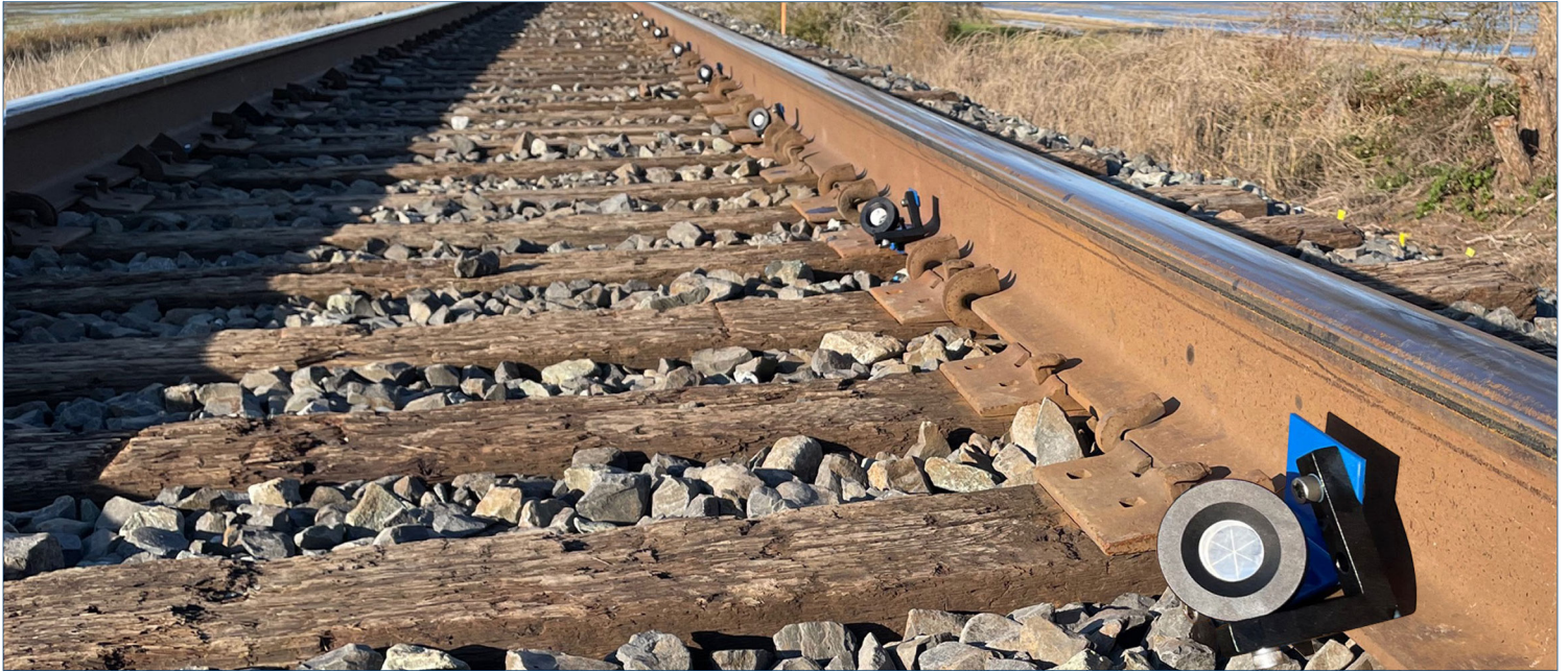
Rail Clip Prisms installed along a 60 foot span of track to monitor for potential settlement
