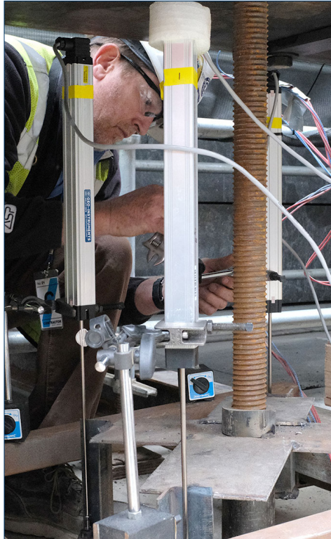
These displacement sensors will be read remotely by the portable logger, so engineers can stay at a safe distance throughout the test.
