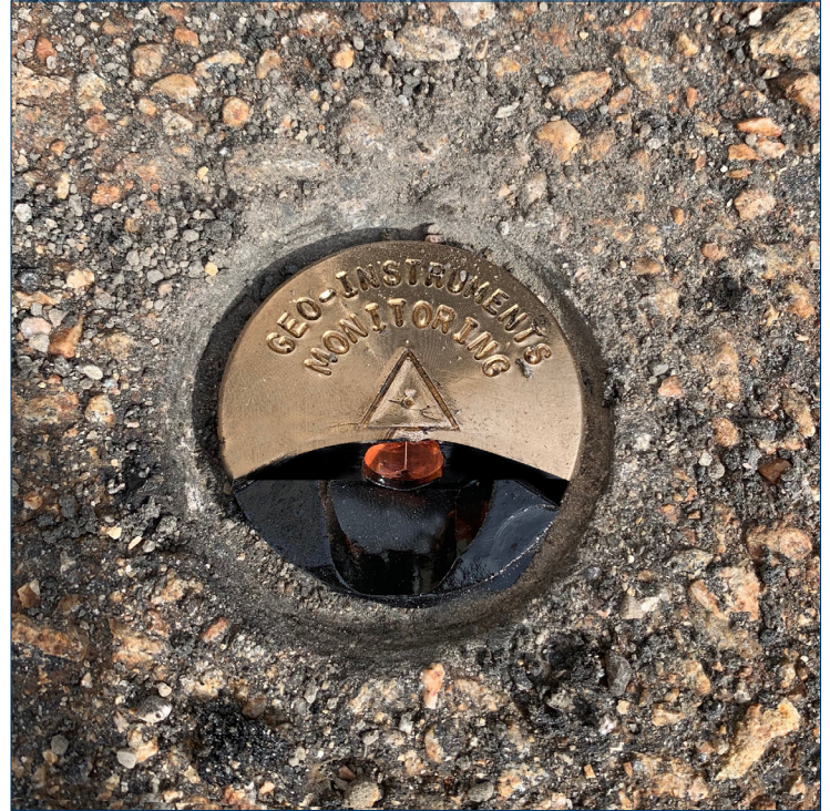
When fully grouted, the monument prism sits flush with the surface.
