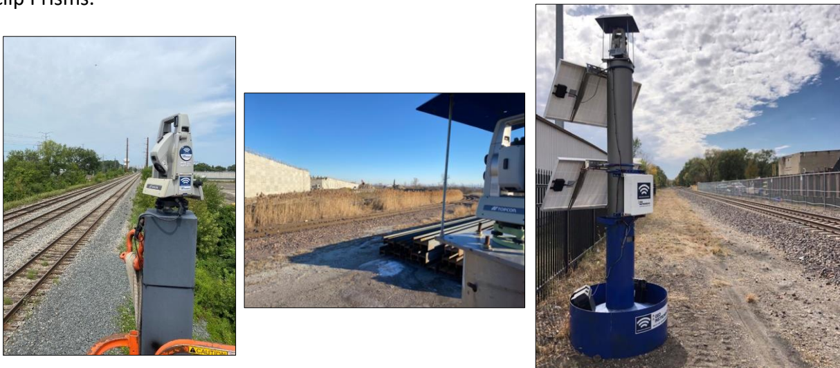
Figure 2. Various AMTS Track Monitoring mounting options.
