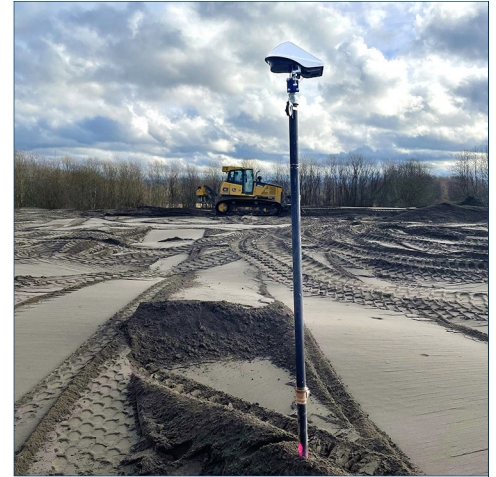
Locator One is ideal for monitoring settlement plates. Radar sensor monitors distance to ground.
