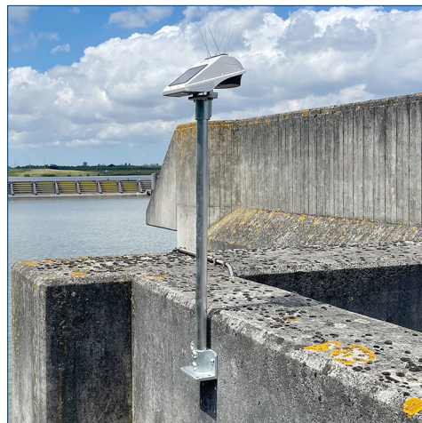
Locator One can be installed on vertical walls if elevated above obstructions.
