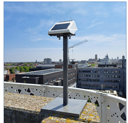
Locator One can monitor structures for adverse effects of tunneling or excavation activity
