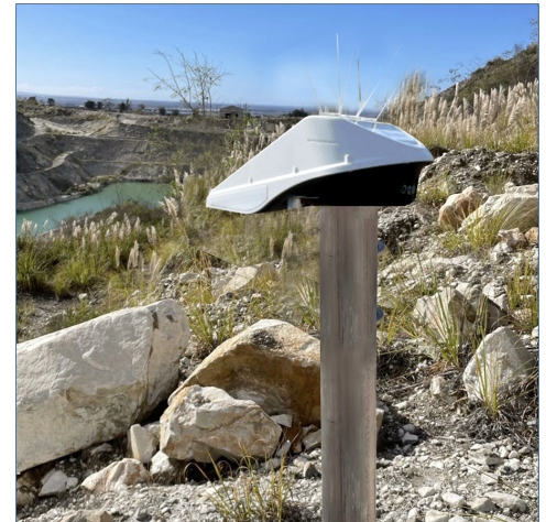
Locator One can monitor slope stability at open pit mines, tailings dams, embankments, and road cuts.
