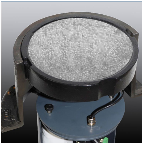
Lid-Link antenna and inspection frame. Cable connects the antenna to the logger package.
