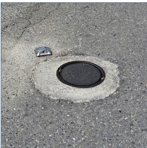
Lid-Link transmits measurements from an instrument installed below the road surface.
