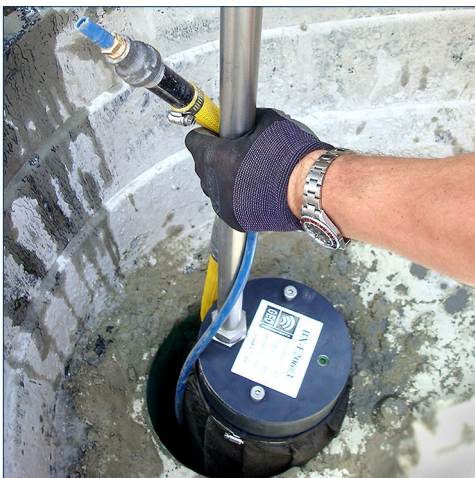
Installation of instrument and logger package.
