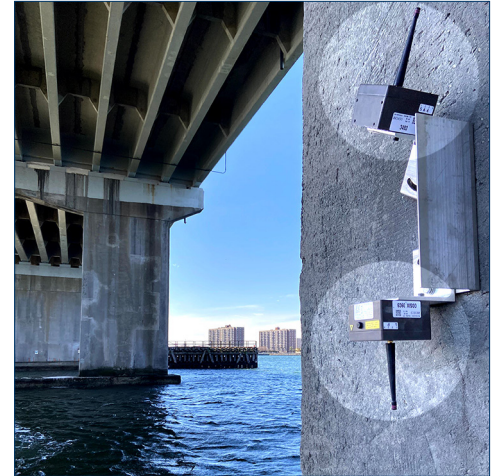
Laser-Tilt sensors monitored the stability of bridge piers while repairs were made to the bumper system.
