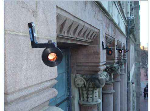
L-Bar Prisms on Building Facade
