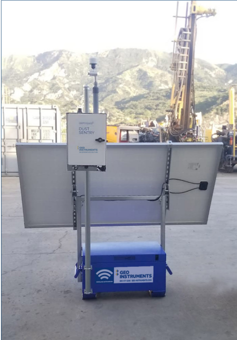
This solar-powered dust monitor is available with wind and noise modules. Measurements are displayed on website and smart phones.
