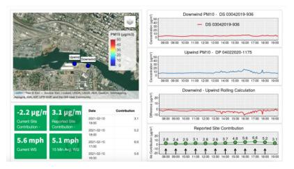
This data was then shared with engineers and stakeholders via a site dashboard. Diagnostic alerts were configured, which sent email and SMS text messages to qualified personnel when triggered. The client could then remotely access control parameters and recalibration tools. This ensured the Dust Sentry systems operated optimally, preserving the accuracy, reliability, and integrity of the air quality data.
