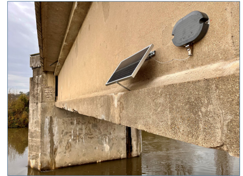
The AD-SIGNUM System provides automated asset monitoring for existing structures such as concrete bridges and dams. Sensors are compact, wireless, self-powered, and simple to install.
