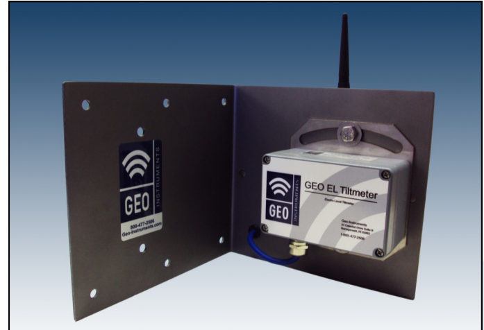
Above: Tiltmeter unit shown on angle bracket (integrated with Wireless Minilogger data logging system). Bracket configuration is designed to allow two tiltmeters installed orthogonally for biaxial tilt measurements.
