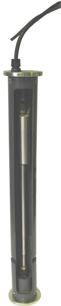
Jointmeter (Cross Section)
