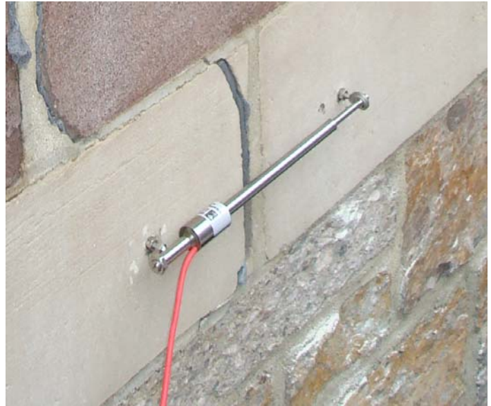
Above: Crackmeter unit shown with standard rebar anchors. Special angle brackets may be provided to allow configuration of three crackmeters in an X Y and Z orientation.
