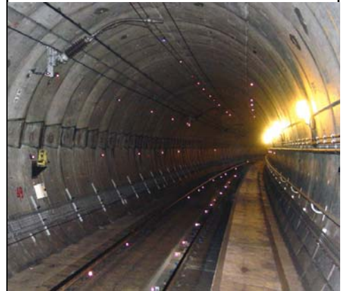
Above: AMTS in tunnel application. Below: Geo-Instruments L-Bar 25.4mm prism can be attached to structure using either hardware or epoxy.
