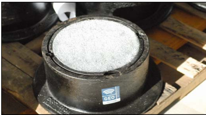
WMPBX Flush mount antenna in its setting frame.
