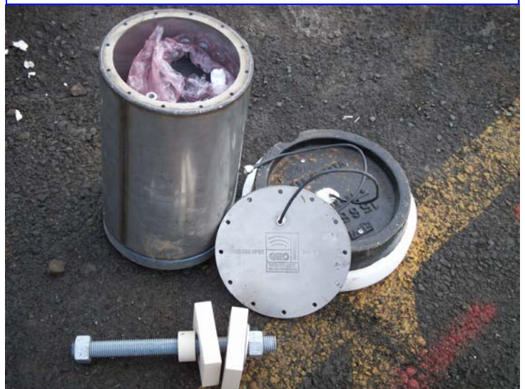
Right: Completed flush mount logger system, below: Flush mount SS lid, and flush antenna (upside down), below, foreground weldments for load cell bearing.
