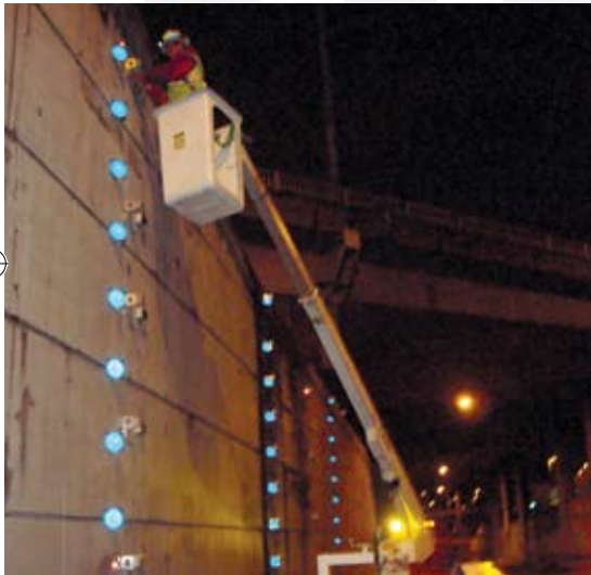
The laser scan targets were made of an aluminum base with circular laser scan reflective areas and a special horizontal angle offset to maintain perpendicularity to the laser scan locations.
